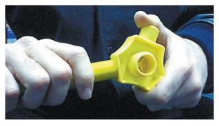
**Step 3** Slide the pipe onto the fitting until it stops. If fitted correctly, the pipe should be visible through both crimp sleeve windows (arrowed below).
