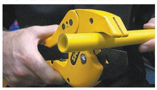
**Step 2** Calibrate pipe with the IPLEX rounding tool. Part No. FK1RNDTOOL.
